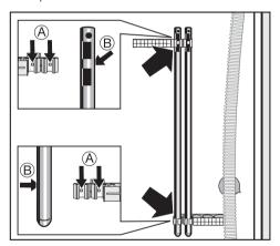
■ Fasten the shipping struts to the rear of the washer. Take care to insert the drill holes correctly, <sup>®</sup>, into the clamps, <sup>®</sup>.
